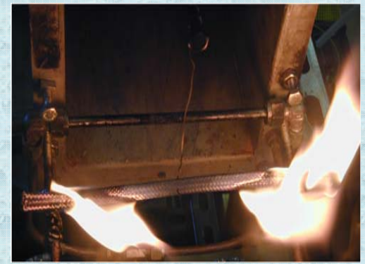
Top view ~185 s after ignition flame spread to the end
