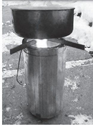
Figure 1: Typical cookstove with pot suspended at three points. (Photograph courtesy of C. Pemberton-Pigott).
