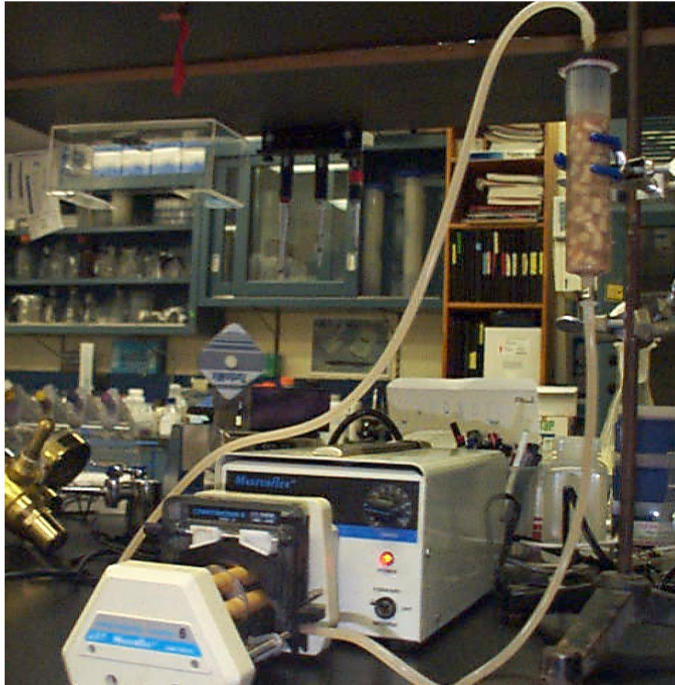
Reaction column with circulation line through a peristaltic pump
